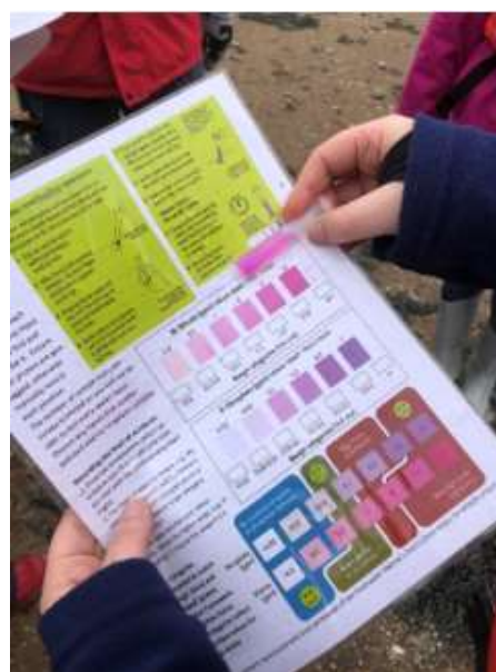
Figure 6: PackTest nitrate testing tube being compared against the colour testing chart provided in the SWEPT survey guidance.
