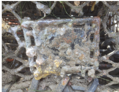
The same 'blank' hatch after 11.5 months. Wire has failed on two sides. Fouling by marine growth evident. (Only hauled twice between November and May).
