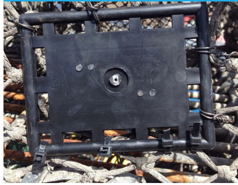
'Blank' hatch example fixed with cable ties (one side) and steel wire (three sides).
