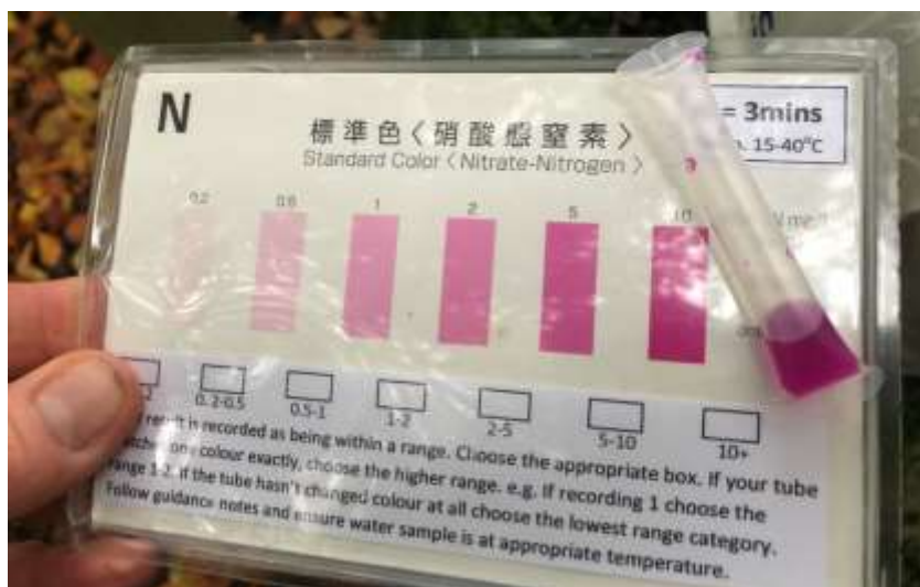
Figure 3: Nitrate analysis card used for identifying nitrate levels in water samples (Richard Vaughan)
